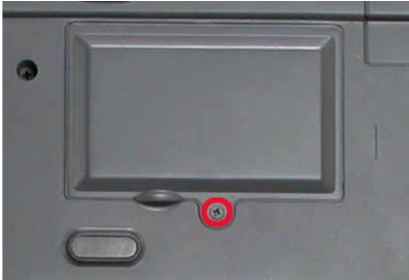
Fig. 6 Removing the screw retaining the memory module slot cover
